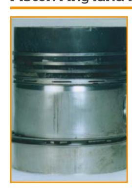
Symptom: Loss of power. Oil consumption. Emission of fumes from engine breather. **Cause:** Leaking injectors or injectors with poor
