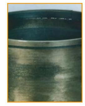
**Symptom:** Combustion gases ventilating to coolant, Engine noise, Eventual destruction of liner. Cause: Incorrect distribution of pressures on liner flange as may be caused by: Cylinder block distortion. Incorrect tightening of cylinder head studs. Misaligned block counter bore. Foreign material assembled under flange.Incorrect location of cylinder head gaskets. Incorrect liner assembly procedures. Incorrect or non-approved gasket. Incorrect reworking of the flange seat, if applicable.
