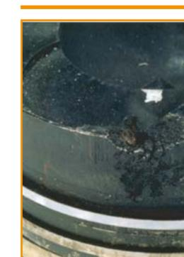
**Symptom:** Loss of power, emission of fumes from engine breather. Exhaust smoke. Cause: Incorrect fuel injection, injection timing, over fuelling, damaged or incorrectly located injector. **Remedy:** Inspect and correct fuel injection equipment and timing. Check and correct any damage to cylinder bore. Replace piston.
