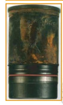
**Symptom:** Loss of coolant. Cause: Incorrect piston to liner clearance, poor seating of the liner in the bore, use of unsuitable coolants, engine operating temp too low.
