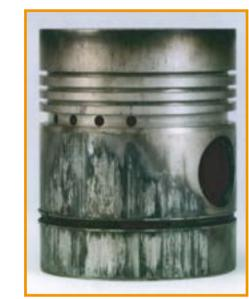
**Symptom:** Loss of power. Engine noise. Fumes from engine breather. Cause: Use of unsuitable liner sealing ring, use of
