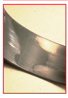
Symptom: Overplate wear only in the crown area of bearing shell towards the edge zones. Worn zones are shifted against each other in circumferential direction. Cause: Centerlines of bearing and journal are not parallel.
