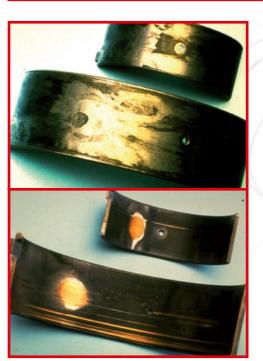
Symptom: Heavy local overplate wear. Local concentration of tin on steel back. Cause: Micro-movement of bearing shell versus housing bore surface due to low pressfit. **Remedy:** Check inner diameter of housing bore. Check cleanliness of housing parting faces. Tighten bearing bolts correctly.
