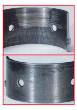
Symptom: Localised surface disruption of bearing surface. The back of the bearing will be marked or indented behind the area of damage. **Cause:** Foreign material assembled between the back
