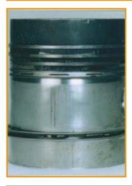
Symptom: Loss of power. Oil consumption. Emission of fumes from engine breather.
