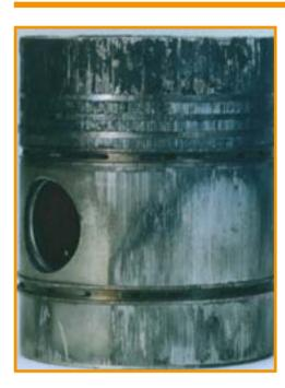
**Symptom:** Loss of power. Engine noise. Fumes from the engine breather.
