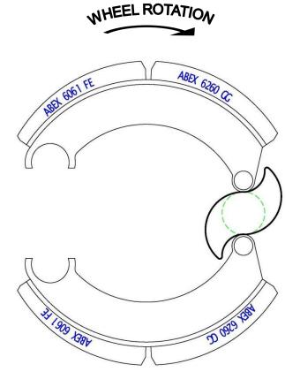
ALWAYS INSTALL ABEX 6260 GG ON THE CAM END OF THE SHOE ALWAYS INSTALL ABEX 6061 FE ON THE ANCHOR END OF THE SHOE
