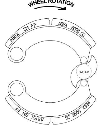
ALWAYS INSTALL ABEX 6098 GG ON THE CAM END OF THE SHOE ALWAYS INSTALL ABEX SM FF ON THE ANCHOR END OF THE SHOE
