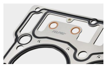
Both of these head gaskets include a patent-pending oversized pushrod guide hole surrounded by a non-abrasive material that protects potential contact areas. This unique feature helps technicians eliminate premature pushrod wear and potential oil contamination caused by pushrod debris entering the engine oil.
