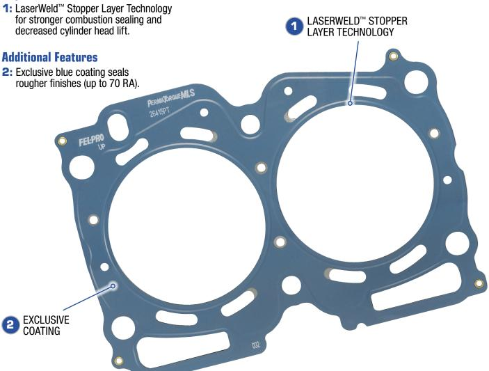
**SALES TIP:** MLS (multi-layer steel) technology is now the industry standard among OEMs, in head gasket design due to the increased casting motion encountered in smaller, lighter and more powerful engines. Counterpersonnel should always sell an MLS replacement head gasket for vehicles originally equipped with MLS gaskets.
