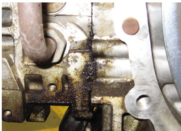
External oil leak from failed head gasket
