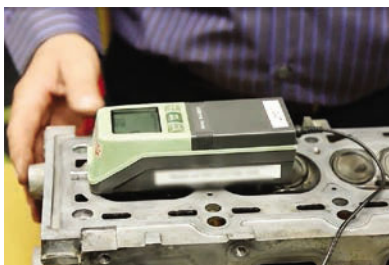
John Gurnig using a handheld profilometer in the Fel-Pro Field Test Garage
