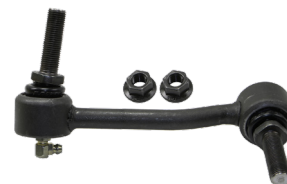
Sway Bar Link Kit – Part No. K750277
