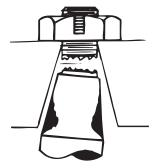
NOTE: THIS KIT MAY CONTAIN SELF TAPPING GREASE FITTING(S) FOR THREADED OR NON-THREADED HOLES. NOTA: CE JEU PEUT COMPRENDRE UN OU DES GRAISSEURS AUTOTARAUDEURS POUR TROUS FILETÉS OU NON FILETÉS. NOTA: ESTE JUEGO PUEDE CONTENER ACCESORIO(S) PARA GRASA AUTORROSCANTE(S) PARA AGUJEROS CON O SIN ROSCA
