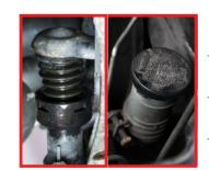
APPEARANCE None or leakage/wet spots at master or slave cylinder
