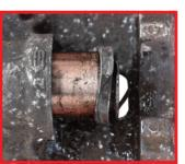
**APPEARANCE** Wet spots around brake caliper
