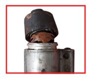
**APPEARANCE** Rust around brake cylinder pins
