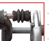
**APPEARANCE** Uneven wear of brake pads on one brake
