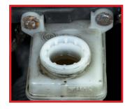
PPEARANCE Abnormal brake pedal behaviour Brown contaminated brake fluid
